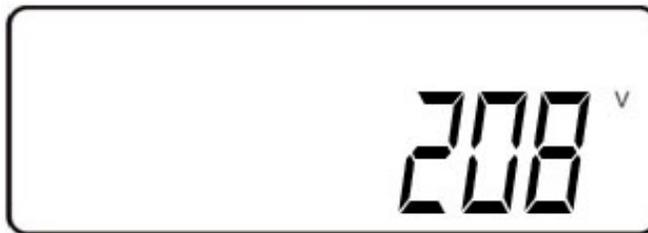
Inverter output voltage set to 208V. Selectable to 200, 208, 220, 230, 240V. This is the voltage sent to the output transformer primary. The UPS output voltages depend on what output configuration is chosen. Please refer to the Output Configuration section of this manual.
