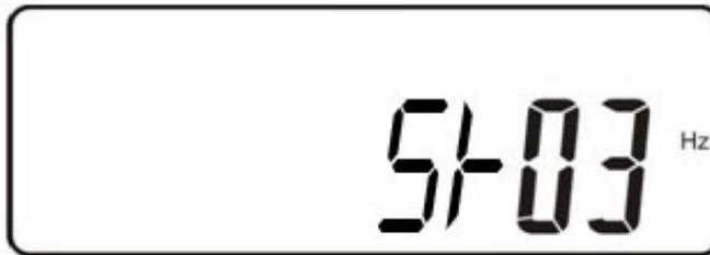
Frequency Window is +/-3 Hz. Selectable to  $\pm 1$ Hz.
