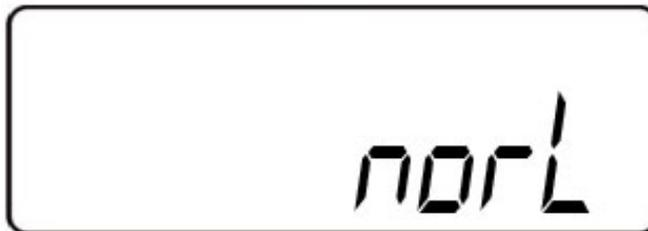
The UPS is operating in "normal mode". Selectable to ECO, CF50, CF60, and Normal.
