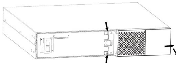
Step 4: Remove the metal top cover of the battery box by unscrewing 8 screws present on the two sides (4 on the right side and 4 on the left side), 3 screws on the top and 4 screws on the back side.
