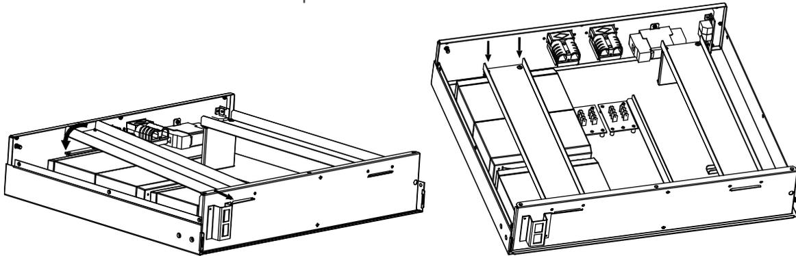
**Note:** To install the second string of batteries, repeat the same procedure on the right side of battery box.
