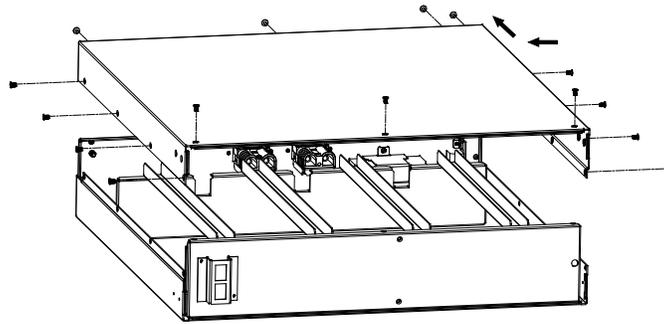
Step 5: Once the battery box is opened, remove the battery hold down brackets present on the left side of the battery box by unscrewing the 2 screws on each bracket.
