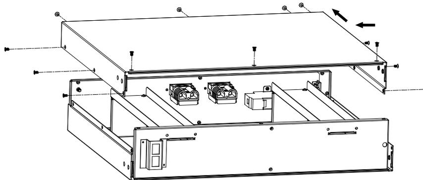
Step 5: Once the battery box is opened, remove the battery hold down brackets present on the left side of the battery box by unscrewing the 2 screws on each bracket.
