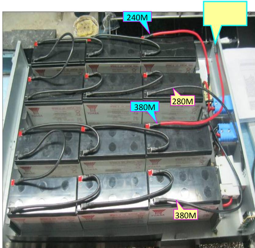
**Note:** The cable connection from the external battery connector to PCB is already present inside the battery box. All the other cable connections should be made in accordance with the above wiring diagram.
