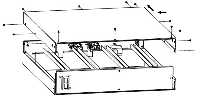
Step 5: Once battery box is opened, remove the battery hold down brackets present on the left side of the battery box by unscrewing the 2 screws on each bracket.
