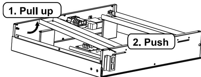
**Note:** To install the second string of batteries, repeat the same procedure on the battery hold down brackets on the right side of the battery box.
