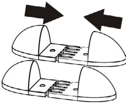
Inter-connect the tower brackets that shipped in the box with the UPS
