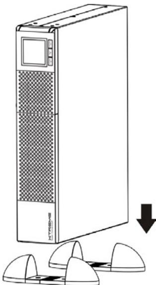
Carefully lower the UPS into the brackets as shown
