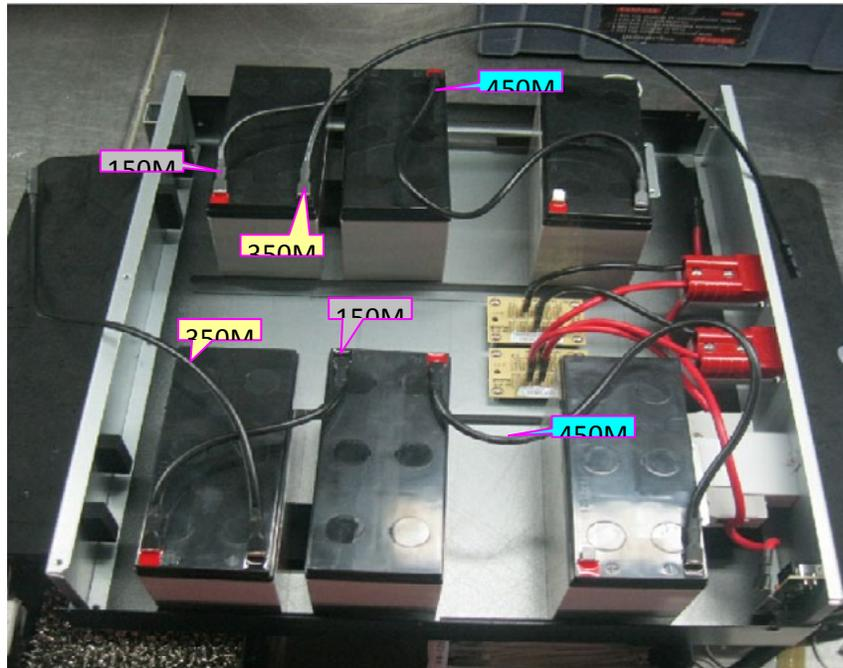
**Note:** The cable connection from the external battery connector to PCB is already present inside the battery box. All the other cable connections should be made in accordance with the above wiring diagram.
