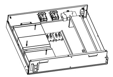
**Note:** To install the second string of batteries, repeat the same procedure on the right side of battery box.
