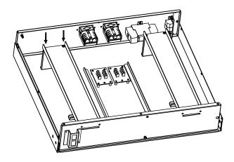
Pull up first and then push the battery fixing plate.
