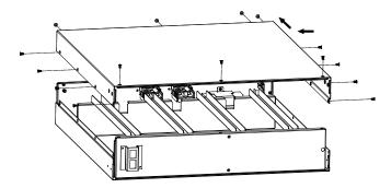
Step 5: Once battery box is opened, remove the battery hold down brackets present on the left side of the battery box by unscrewing the 2 screws on each bracket.
