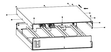
Step 5: Once the battery box is opened, remove the battery hold down brackets present on the left side of the battery box by unscrewing the 2 screws on each bracket.
