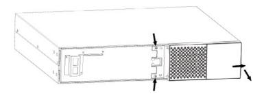
Step 4: Remove the metal top cover of the battery box by unscrewing 6 screws present on the two sides (3 on the right side and 3 on the left side), 3 screws on the top and 4 screws on the back side.
