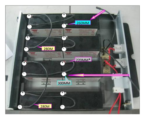
**Note:** The cable connection from the external battery connector to PCB is already present inside the battery box. All the other cable connections should be made in accordance with the above wiring diagram.
