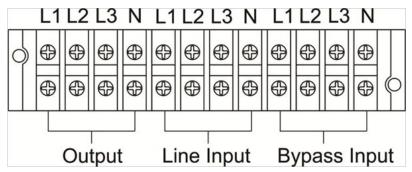
Terminal Block wiring diagram of GT90-20K(L)
