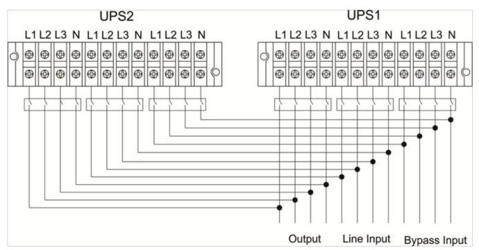
Wiring diagram of parallel system for GT90-20K(L)
