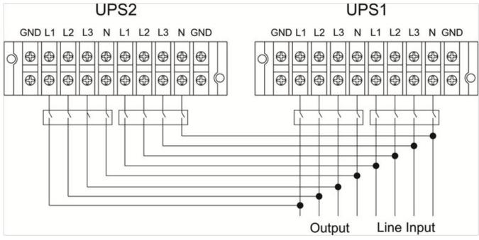
Wiring diagram of parallel system for GT90-30K(L)
