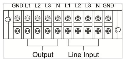
Terminal Block wiring diagram of GT90-30K(L)
