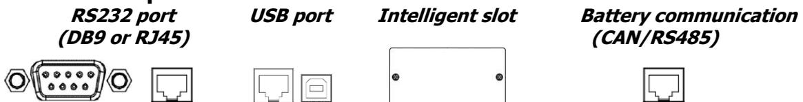
To allow for unattended UPS shutdown/start-up and status monitoring, connect the communication cable one end to the USB/RS-232 port and the other to the communication port
