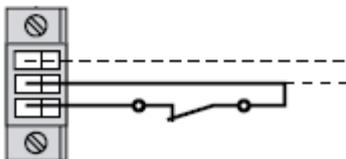
**Contact open:** UPS shuts down and Fault LED will be ON.
