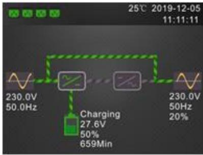
NOTE: While the UPS is operating, the LCD will dim and display a screen saver if there is no active alarm or user interaction for two minutes. After 5 minutes, the screen will turn off. Any button press will wake it. If an alarm or fault occurs or if any button is pressed, the UPS-flow screen displays.
