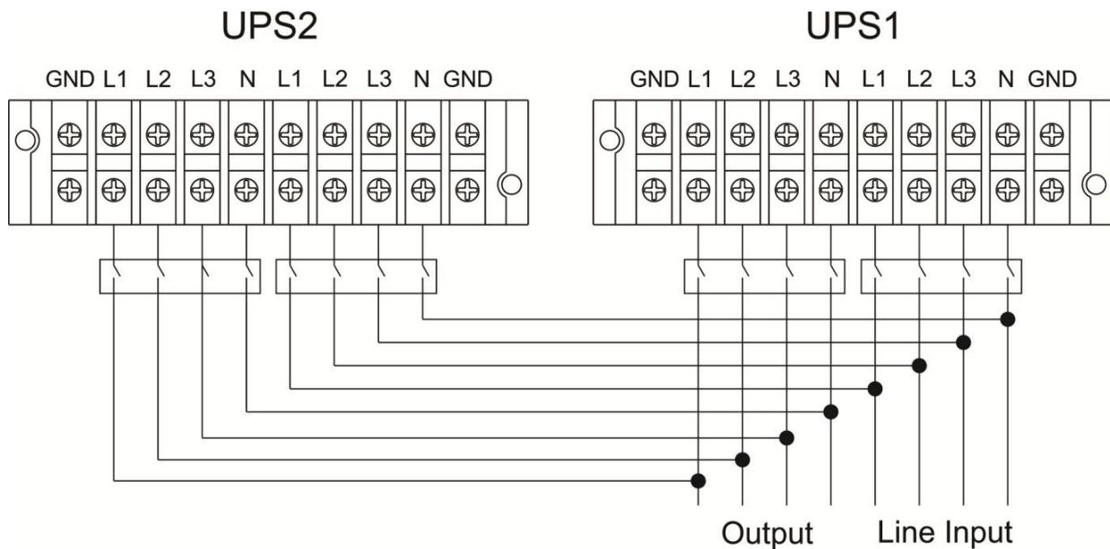
Wiring diagram of parallel system for 30K(L)
