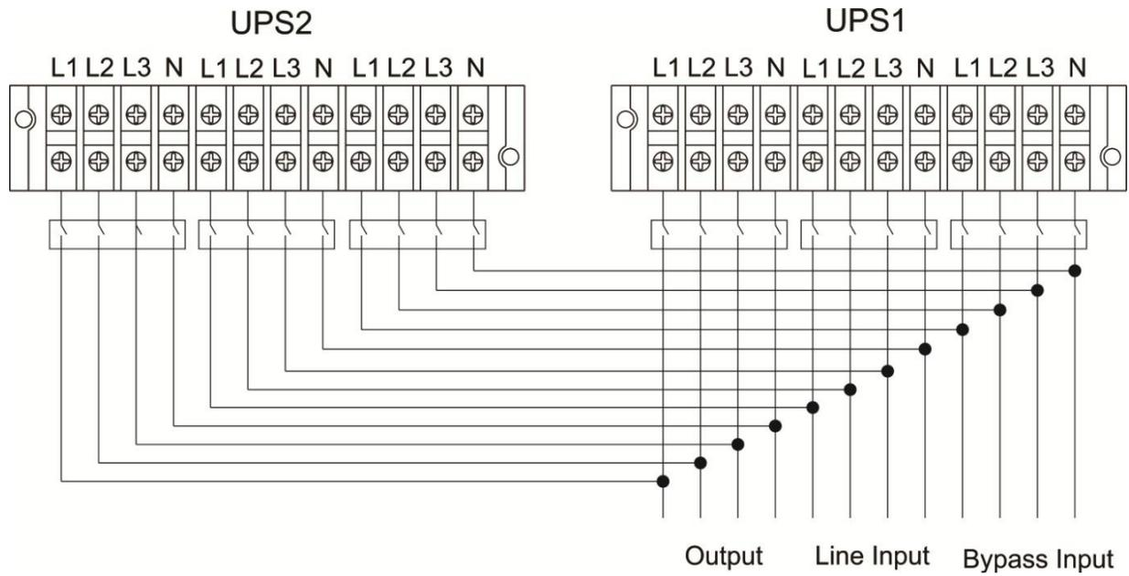
Wiring diagram of parallel system for 20K(L)
