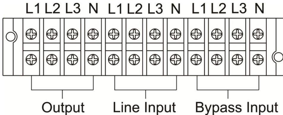
Terminal Block wiring diagram of 20K(L)
