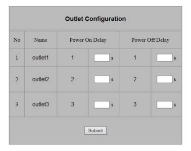
The control action include "on immediate", "on delay", "off immediate", "off delay" 4 types. "Delay on/off" action is only available after setting the delay time parameter.
