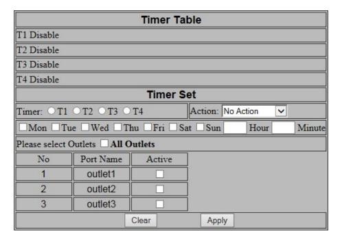
**Timer Table/Timer Set:** User can enter up to 4 preset timers. Time is in 24 hour format. Timers can be set for individual or all outlets. To clear the set parameters for T1, T2, T3, or T4: select the desired preset under Timer (T1, T2, T3, T4) and enter "0" in Hours and "0" in Minute and click "Apply". Note: make sure "No Action" is selected in the Action menu.
