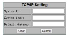
You have to fill in all the information for system IP, system mask and system gateway. When finished it, reboot smart PDU, the new IP address can be used.
